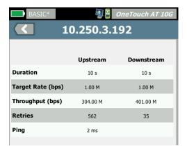
Figure 70. iPerf TCP Test Results
