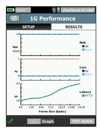
Figure 43. Wired Performance Test Results RFC 2544 sweep, Graphical View Target Rate (bps) is the requested bit rate from the SETUP tab.
