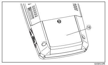
Figure 9. Battery Compartment
