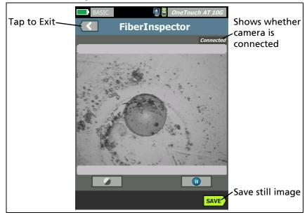
Figure 72. FiberInspector Image of an Endface
