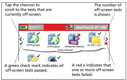
Figure 24. Seeing Off-Screen Tests
