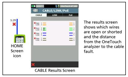
Figure 27. Unterminated Cable with Shorts and Opens
