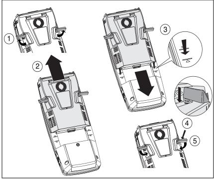
Figure 2. Remove and Install a Module
