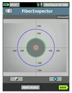
Figure 73. FiberInspector Image with Measurement Scales (fiber with 50  $\mu$ m core shown)
