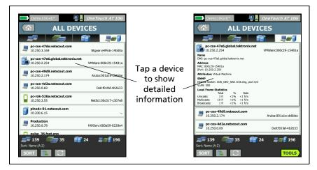
Figure 55. Displaying Wired Device Details
