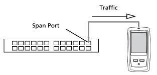
Figure 82. Single-Ended Packet Capture
