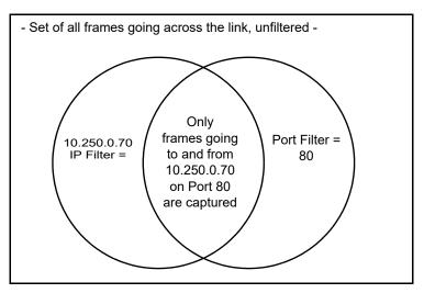
Figure 81. Capture Filters - Logical AND Operation
