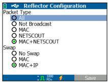
MAC + NETSCOUT - This filter setting allows the LinkRunner to only reflect frames when the destination MAC address field matches the LinkRunner's own MAC address and NETSCOUT payload.
