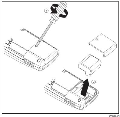
Figure 95. Remove and Install the Battery
